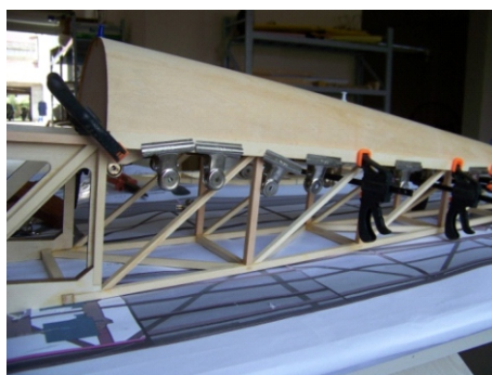
(12) Glue the cover board and fix it with wood sheet to make it more flat.
