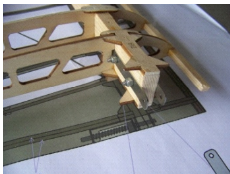
(6) Mark the place of center line and then bore 3mm holes according to the holes of metal parts. And install the metal parts.
