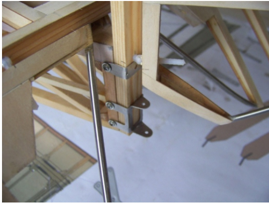
(1) Make the metal parts and install the tail wheel.
