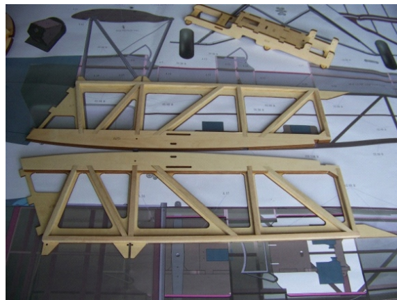
(2) Glue the fuselage lateral plate and the strengthening battens.
