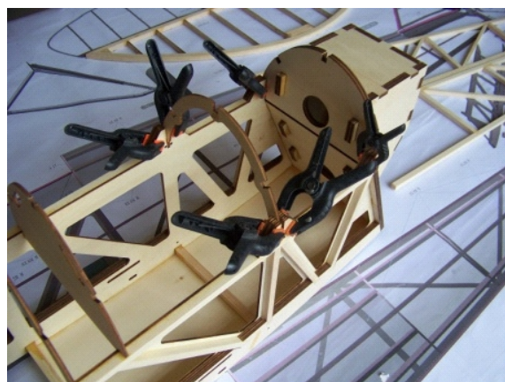
(6) Glue the bulkhead A8, A12, A13 and strengthening plate A39.
