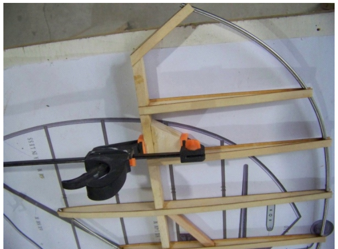
(4) Joint and glue the stainless steel tube and framework. And then glue the strengthening plate.
