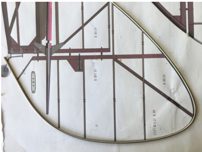
(3) Bending the 4mm stainless steel tube.
