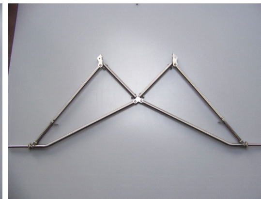
(3) Joint the spring & sliding sleeve, and lock with each end of nuts, then insert it to steel tube and the connection, keep the shaft movable. (4) Fix the damper on the wheel shaft with screw.
