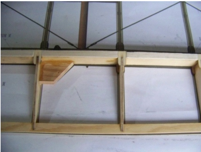
(14) Joint the strengthening plate for servo horn.
