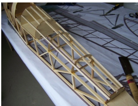
(11) Joint and glue the bulkhead and battens according to the installation drawing.
