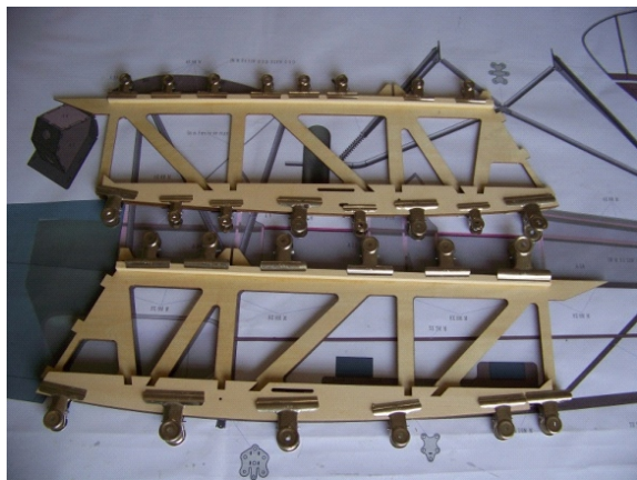
(2) Glue the fuselage lateral plate and the strengthening battens.
