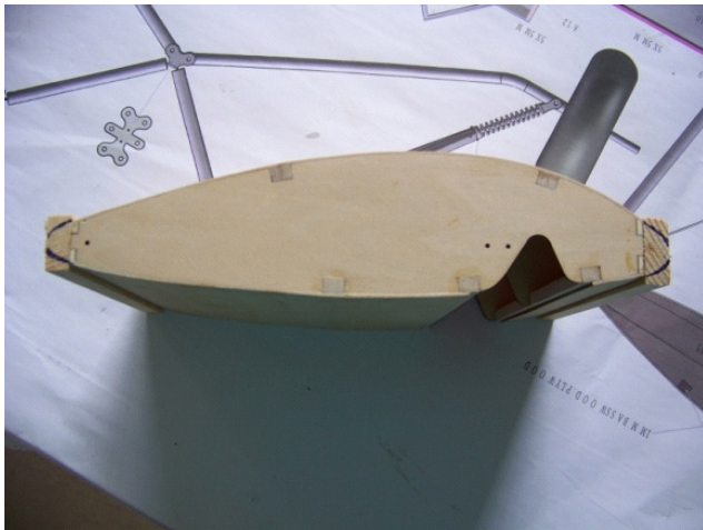
(2) Glue the wood bricks on the front (wider) and back (narrow), and then trim them to be cambered.
