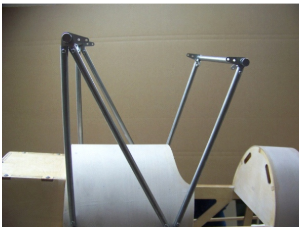
Supporting for the fuel tank.
