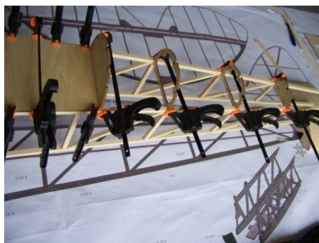
(11) Joint and glue the bulkhead and battens according to the installation drawing.
