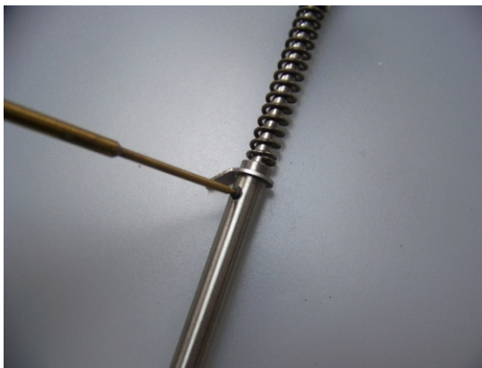
(3) Joint the spring & sliding sleeve, and lock with each end of nuts, then insert it to steel tube and the connection, keep the shaft movable. (4) Fix the damper on the wheel shaft with screw.
