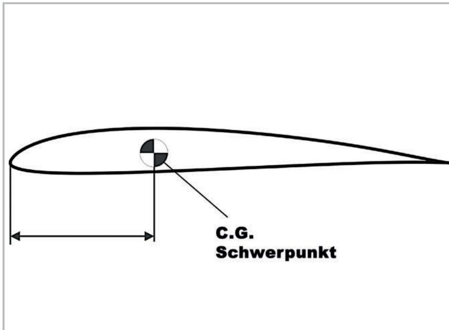
Finally, the model must be assembled, the propeller properly mounted and tightened to achieve the required **center of gravity of 74 mm**. The center of gravity can be adjusted by changing the battery position.
