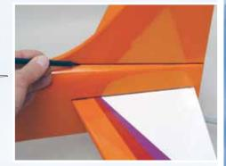
the right. Install the fin and then mark the tailplane on the top and bottom where it enters the fuselage using a soft, water-soluble pen. Repeat for the fin as shown.
